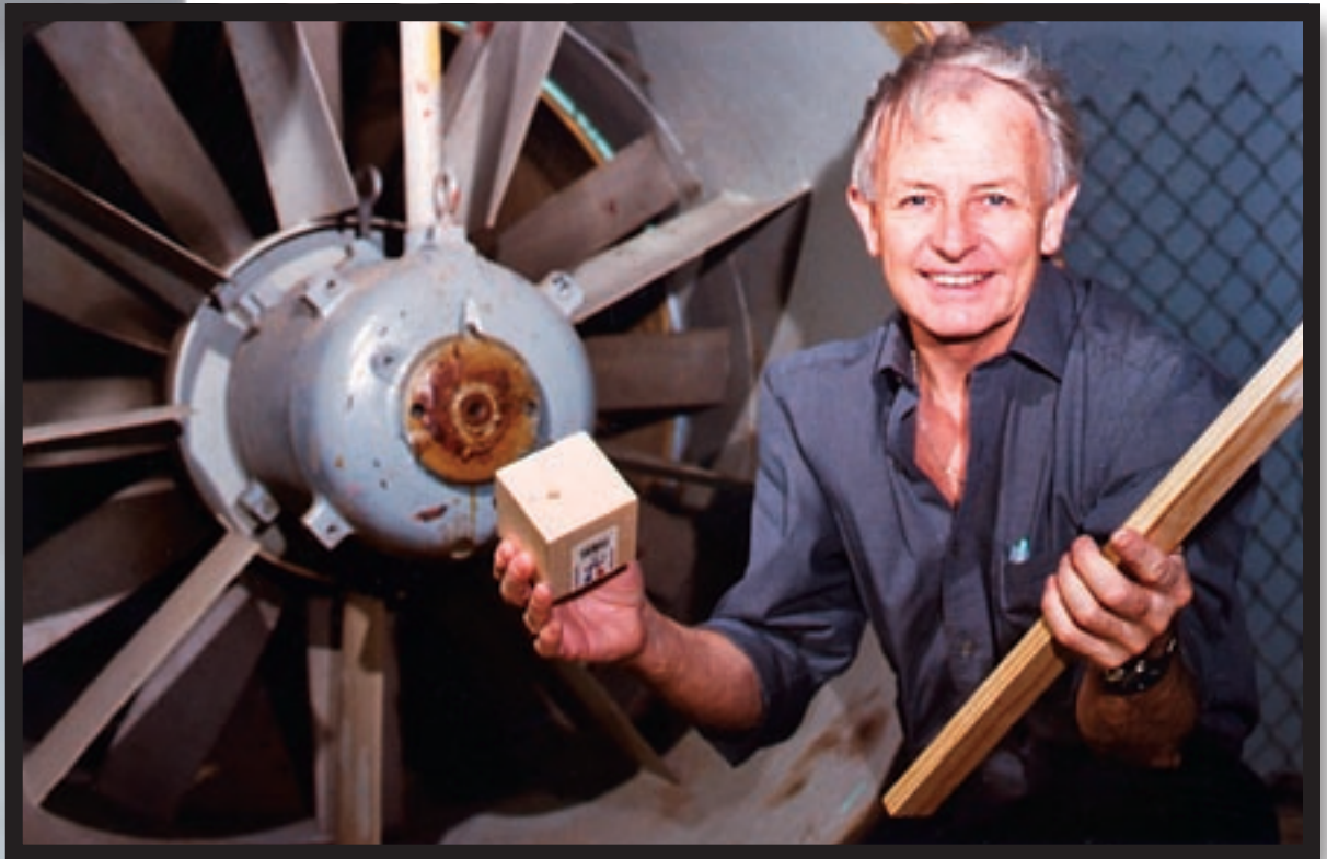
John Holmes shows the wooden forms he used to study windborne debris near the large fan that drives the wind tunnel in his experiments. Photo by Paula Ouder.
